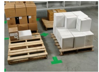
3. Colour-code material storage areas.
