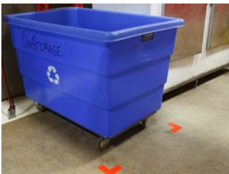
4. Colour-code non-material storage fixtures.
