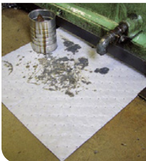
MRO pads under leaking seals & faucets. Ideal to catch small drips.
