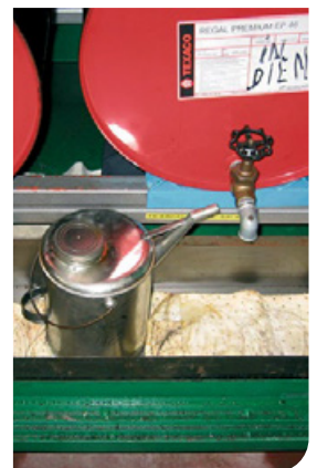
OP pads under oil cans & drums to catch small drips.
